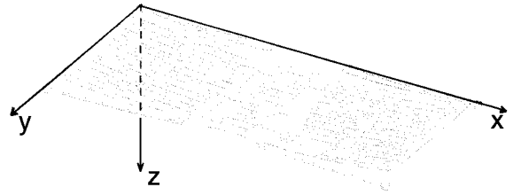
Fig. 10. Simulated warped switch structure (by SUGAR). The maximum switch deflection is approximately 23 \mu\text{m} .
